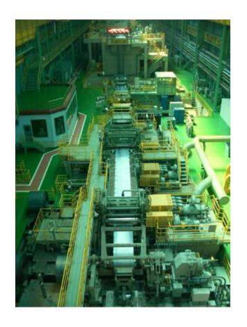
Hot rolled black is uncoiled and sent through a series of hydrochloric baths that removes scale, rust, and unwanted debris. The coil is then lightly oiled for temporary rust prevention.
